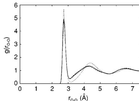
FIG. 4. Oxygen-oxygen site-site distribution function for HDA ( $I_h$ ) (solid line), HDA(VII) (dashed line), HDA(VIII) (short dashed line), liquid water cooled from 270 to 135 K at 1 bar (path 1) (dotted line), and liquid water cooled via path 2 (dot-dashed line).
