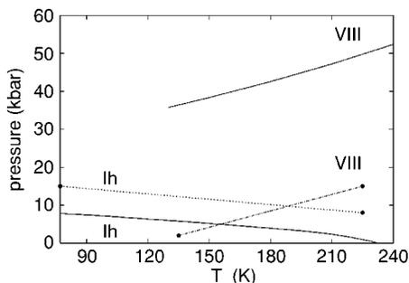
FIG. 7. Extension of the thermodynamic equilibrium melting curves (solid lines) along with the limits of stability obtained by changing the pressure along isotherms, both for ice  $I_h$  (dotted line) and ice VIII (dot-dashed line).
