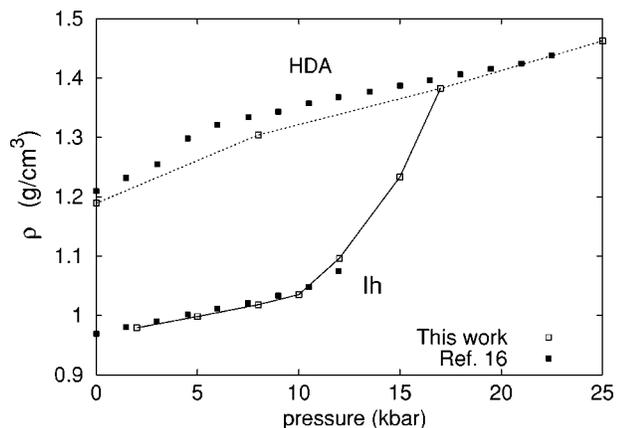
FIG. 3. Comparison for  $T=77$  K between Monte Carlo results of this work ( $\square$ ) with data from molecular dynamics simulations ( $\blacksquare$ ) of Martoňák, Donadio, and Parrinello (Ref. 16). Solid line ice  $I_h$  equation of state. Dashed line HDA equation of state.
