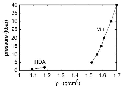
FIG. 1. Equation of state for ice VIII at 135 K. Dashed line is the HDA branch, solid line is the ice VIII branch.
